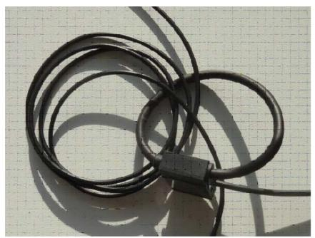
Sensitivity is 5 times higher if the power cable is wrapped around the coil 5 times
