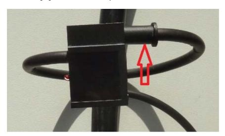
**NOTE:** The sensor is not sensitive to power direction.
