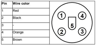
M12 5 Pin female connections (internal, back side)
