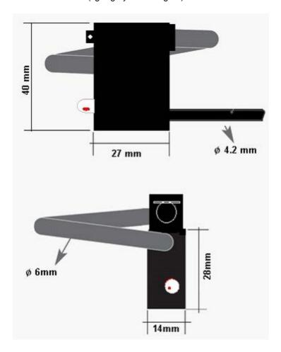
The hole (?1.5mm) in the plug can be used to seal the device.
