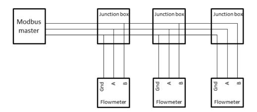
Shielded twisted pair should be used. For Modbus field cabling only use the <u>recommended cables</u> sized and shielded in line with the specific situation in your plant. Connection of a third wire between the master and slave should be done to limit the common mode voltage that can be impressed on the slaves inputs. The cable shielding should only be connected at the earth rail in the VPVision cabinet. The cable shielding should not be connected to any other earth connection point.
